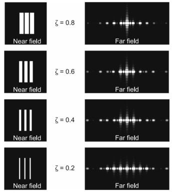
An increase in the duty cycle leads to a reduction in the number of high-peak-intensity nodes, as well as an increase in the energy concentration in the central diffraction spot.
