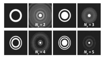
Increasing the number of zones progressively reduces the width, as well as increases the peak intensity and the total power contained in the central peak of the diffraction pattern.
