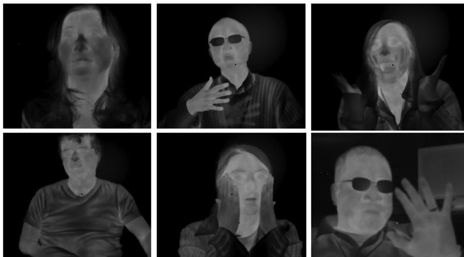
Figure 17.8 A set of images taken with a 320 \times 256 format LWIR CBIRD FPA operating at 78 K.
