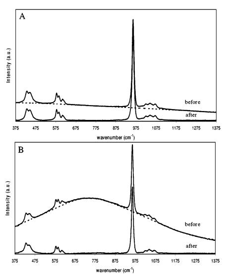
**Fig. 3** Representative Raman spectra illustrating the background fluorescence acquired from (A) the majority of sound and carious dental enamel and (B) from a few number of carious sites. For both panels, the upper solid traces illustrate the original spectrum. The dashed traces are the sixth order polynomial fits that were used for correction and the lower solid traces are the results after subtracting the polynomial fits of the background fluorescence.
