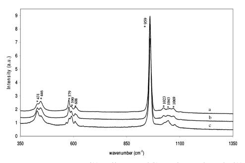
Fig. 5 Representative microspectroscopic Raman spectra of (a) sound human enamel, (b) carious human tooth enamel and (c) synthetic hydroxyapatite (OHAp) acquired with  $\times 10$  objective. Spectra are offset for clarity. The asterisks indicate peak positions. See discussion for further details.
