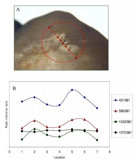
**Fig. 12** (A) Photomicrograph of a tooth surface containing two carious lesions (white areas). Shaded dots represent actual Raman sampling locations with a fiber-optic Raman probe. (B) Intensity ratio plot of various Raman peaks (431, 589, 1042, and 1070  $\text{cm}^{-1}$ ) relative to the 961  $\text{cm}^{-1}$  peak corresponding to the sampling locations shown in (A).
