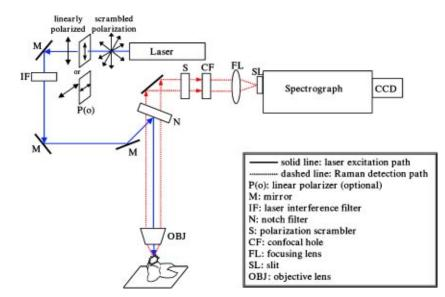
**Fig. 1** Schematic diagram of the Raman microspectroscopic system illustrating the laser excitation (solid line) and Raman signal detection (dashed line) paths for acquiring tooth spectra in a 180° geometry. Abbreviations are provided in the inset for each optical element. The linear polarizer (P) is only used when performing polarized Raman experiments.
