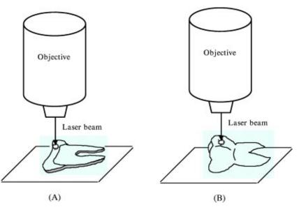
Fig. 2 Diagrammatic representation of the two spectral acquisition configurations using (A) transverse excitation/detection on a longitudinally sectioned (crown to root direction) tooth, and (B) normal excitation/detection on an unsectioned whole tooth. Drawing illustrates the actual sample orientation under the microscope objective.
