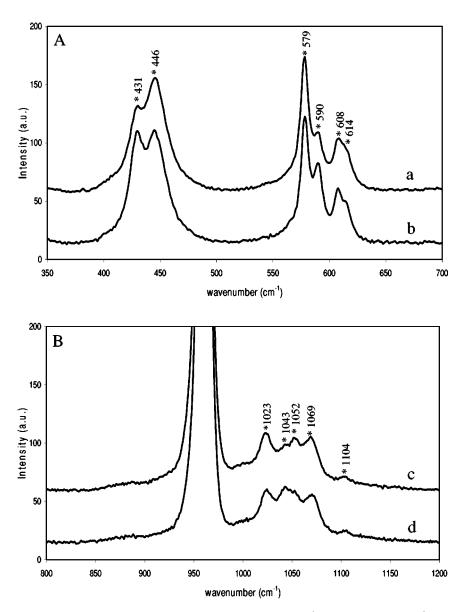
**Fig. 6** Representative microspectroscopic Raman spectra in the region of (A)  $350-700 \text{ cm}^{-1}$  and (B)  $800-1200 \text{ cm}^{-1}$  of sound enamel (a and c) and carious enamel (b and d). Spectra were acquired with  $\times 10$  objective and offset for clarity. The asterisks indicate peak positions.
