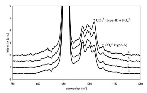
Fig. 11 Representative Raman microspectroscopic spectra in the 750–1200 cm<sup>-1</sup> region of sound enamel measured with (a)  $\times$ 5, (b)  $\times$ 10, (c)  $\times$ 50 and (d)  $\times$ 100 microscope objectives.
