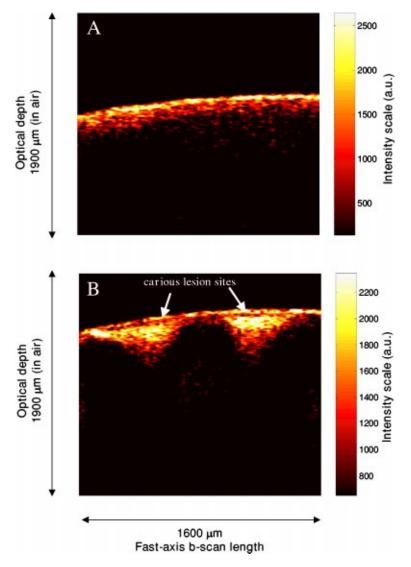
Fig. 4 Representative false-color OCT images of lateral scan length as a function of depth from (A) sound enamel tooth surface (minimum light back scattering with depth) and (B) carious enamel surface containing two lesions (significant light backscattering). The carious lesion sites are indicated with the arrows.
