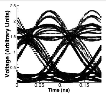
Fig. 3 Eye diagram of voltage corresponding to received current of worst channel after 800 km of propagation with no dispersion compensation.
