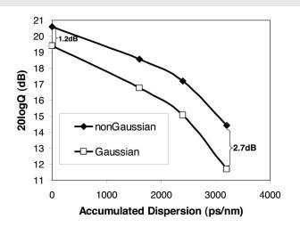
**Fig. 2** System performance in  $20 \log Q$  (in decibels) versus accumulated dispersion (in picoseconds per nanometer).
