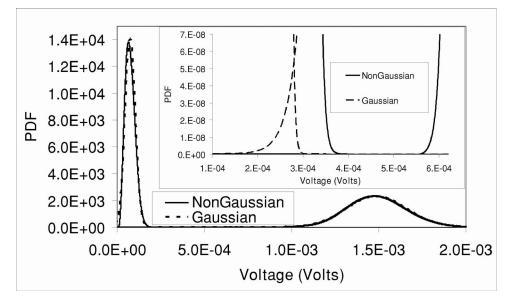
Fig. 4 Graph of pdfs of voltage corresponding to received current from Gaussian assumption (dashed) and non-Gaussian calculation (solid).
