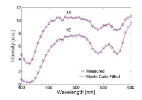
Fig. 2 Calibrated measured and MC-fitted tissue phantom spectra.
