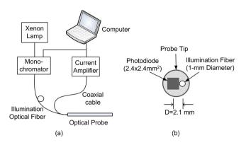
Fig. 1 Schematic of (a) modified spectrometer and (b) probe tip.
