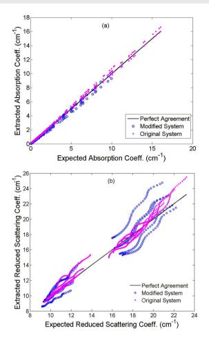
Fig. 3 Extracted versus expected (a) absorption coefficient and (b) reduced scattering coefficient.
