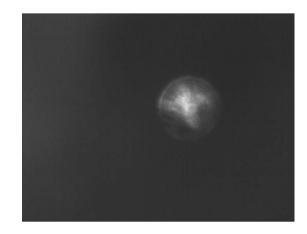
Fig. 2 Image of an attenuated beam that was used as reference image.
