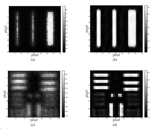
Fig. 5. Estimated ranges for simulation targets: (a) No processing - three bars, (b)  ${\rm GEM_o}$  processing - three bars, (c) No processing - Many bars, and (d)  ${\rm GEM_o}$  processing - Many bars. Utilizing the  ${\rm GEM_o}$  algorithm, simulation results show the image quality improvement and improved range estimation ( RMSE improves 75% for 3 bar target).
