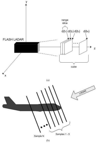
Fig. 1. (a) 3D view of LADAR system model in Cartesian coordinates with each data cube having dimensions of pixel  $\times$  pixel  $\times$  time sample. The variable  $d(t_k)$  corresponds to the  $k^{th}$  receiver detected range image with  $k \in [1, N]$ . (b) Another view of the 3D FLASH LADAR operation. Each range image's full field of view (FOV) is  $128 \times 128$  pixels with a range gate near 2 nanoseconds corresponding to the 3D FLASH LADAR system used for experimental collects.
