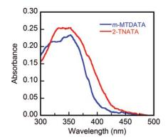
Fig. 3 Electronic absorption spectra of vapor-deposited films of m-MTDATA (30 nm) and 2-TNATA (30 nm).
