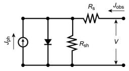
Fig. 4 Equivalent circuit of OPV devices.
