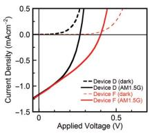
**Fig. 5**  $\mathcal{J}$ -*V* characteristics of device D and device F in the dark and under AM1.5G illumination at an incident light intensity of 100 mW cm<sup>-2</sup>.
