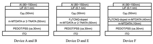
Fig. 1 Structures of fabricated devices.
