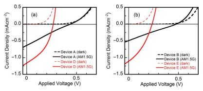
**Fig. 2** J-V characteristics of (a) device A and device D, and (b) device B and device E in the dark and under AM1.5G illumination at an incident light intensity of 100 mW cm<sup>-2</sup>.
