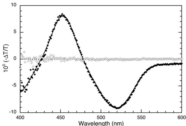
**Fig. 2** EM spectrum of an ITO/HIL/(40 nm) $\alpha$ -NPD/(40 nm)Alq<sub>3</sub>/LiF/Al device, measured at  $-0.7$  V dc bias and with a 0.5 V rms reference bias modulated at 1 kHz. In-phase: filled symbols. Quadrature: open symbols. The line is shown as a guide for the eye.
