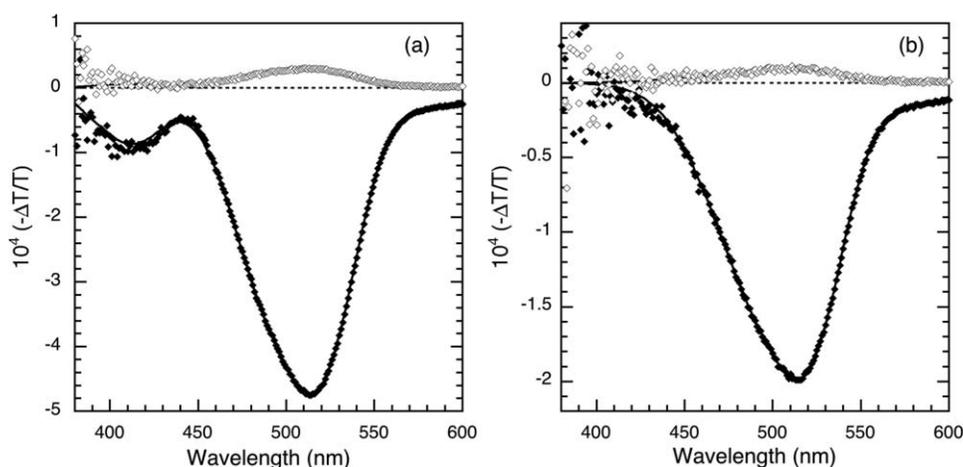
**Fig. 4** EM spectra of the bi-layer OLED measured at (a) 1.7 V dc bias with a reference bias of 0.5 V rms and (b) 3 V dc bias with a reference bias of 200 mV rms. The reference bias was modulated at 1 kHz for both scans In-phase: filled symbols. Quadrature: open symbols. The line is shown as a guide for the eyes for the near-UV portion of the spectrum.
