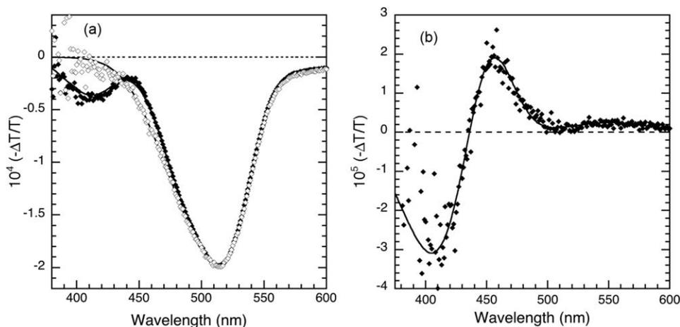
**Fig. 6** (a) EM spectra of the bi-layer OLED from Fig. 5, scaled to the maxima of the  $\alpha$ -NPD<sup>+</sup> peak. Filled symbols: measured with 1.7 V dc bias. Open symbols: measured with 3 V dc bias. (b) The difference spectrum between these two EM spectra.
