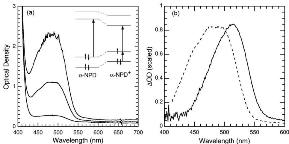
**Fig. 5** (a) Absorption spectrum of a 17 mM  $\alpha$ -NPD solution as it is progressively doped by  $\text{FeCl}_3$ . Inset: a Jablonski diagram of the optical transitions of  $\alpha$ -NPD and  $\alpha$ -NPD $^+$ . (b) Dashed line: doping-induced absorption spectrum of  $\alpha$ -NPD. Solid line: difference between the EA spectrum of a single layer  $\text{Alq}_3$  device and that of the bi-layer device with a PTT:PPFSA hole injection layer.
