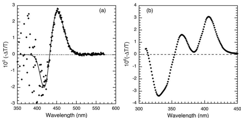
**Fig. 1** EM spectrum of (a) ITO/(100 nm)Alq<sub>3</sub>/Al ( $F = X$  kV/cm) and (b) ITO/(100 nm)a-NPD/Al devices ( $F = 21$  kV/cm). Symbols show the experimental data in (a) and the line shows a multi-Gaussian fit to  $\Delta T$ . The data for Fig. 1(b) was measured by Rohlffing et al. (Ref. 24).
