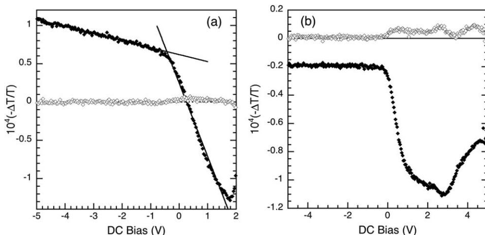
**Fig. 3** Dependence of the (a) Alq<sub>3</sub> EA signal ( $\lambda = 460$  nm) and (b) EM signal ( $\lambda = 520$  nm) on the applied bias. The reference voltage was 0.2 V rms, modulated at 1 kHz for both measurements.
