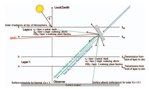
Fig. 3 Schematic of the radiative transfer geometry in the Remote Observer Scenario Toolkit.
