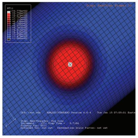
**Fig. 6** Example target thermal response from ABAQUS for a cylindrical test object with a surface temperature of 300 K illuminated by a laser spot with a Gaussian distributed irradiance profile. Facet size is 5 mm.
