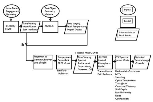
Fig. 2 Schematic of the CDE Remote Observer Scenario Toolkit.
