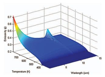
Fig. 7 Wavelength and temperature dependent emissivity for bare aluminum.
