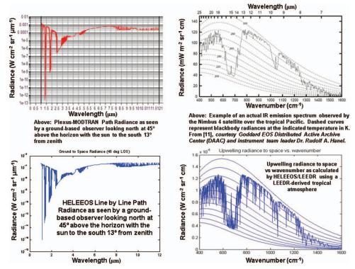
**Fig. 4** Upper left: MODTRAN radiance for a 45° LOS in a mid-latitude atmosphere with maritime aerosols. Lower left: HELEEOS radiance for a 45° LOS in a mid-latitude atmosphere with maritime aerosols. Upper right: IR emission spectrum as measured by NIMBUS 4 over the Tropical Pacific, courtesy of Ref. 11. Lower right: HELEEOS/LEEDR 1000-pt calculated IR emission to space from a LEEDR-derived tropical atmosphere; blackbody curves are the same as those in the upper right.
