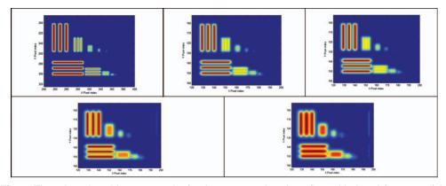
**Fig. 8** Three bar chart blur test results for the 5 sensor bands, reflected in-band (1.315  $\mu$ m) in upper left, MWIR 1 (3.9  $\mu$ m) upper center, MWIR 2 (4.7  $\mu$ m) upper right, LWIR 1 (8.0  $\mu$ m) lower left, LWIR 2 (10  $\mu$ m) lower right. At the shortwave infrared wavelength results are dominated by turbulence and detector size, while at the longer wavelengths diffraction effects dominate.
