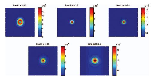
**Fig. 10** Photoelectron images for 5 bands, reflected in-band (1.315  $\mu$ m) in upper left, MWIR 1 (3.9  $\mu$ m) upper center, MWIR 2 (4.7  $\mu$ m) upper right, LWIR 1 (8.0  $\mu$ m) lower left, LWIR 2 (10  $\mu$ m) lower right. Associated sensor video captures time- and wavelength-dependent spot morphology with degradations due to atmospheric transmission and path radiance effects over 5 s following laser initiation. (wmv, 343 KB) [URL: http://dx.doi.org/10.1117/1.3626025.2].
