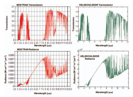
**Fig. 5** Left-hand plots: MODTRAN transmission and path radiance plots for the 45° LOS from the observer to target for the atmosphere used in this study. Right-hand plots: HELEEOS/LEEDR transmission and path radiance plots for the 45° LOS for the Vandenberg atmosphere.
