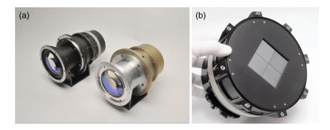
**Fig. 3** (a) Two lens prototypes were constructed during phase A. One was subjected to thermal vacuum testing at the operational temperature; the other was subjected to vibration testing. (b) The detector assembly of one of the prototype lenses. The frame-store regions of the CCDs are covered.
