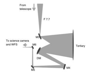
Fig. 7 SMT optical layout replacing the FSM with a deformable mirror on a gimbal.<sup>15</sup>
