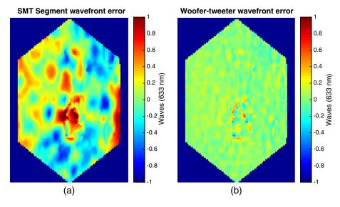
Fig. 12 (a) SMT RMS wavefront error 0.32 waves and (b) SMT woofer-tweeter wavefront error 0.07 waves using 471 actuators.
