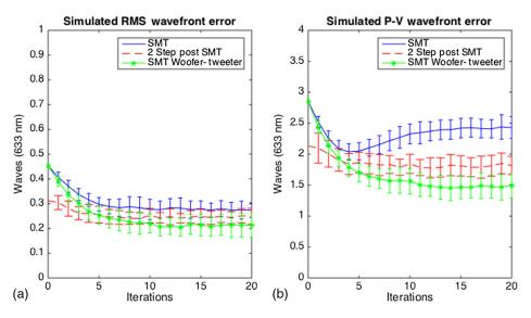
Fig. 14 Simulated SMT and SMT woofer-tweeter wavefront error history using an iterative constrained minimization controller, (a) RMS wavefront error and (b) peak-to-valley wavefront error.
