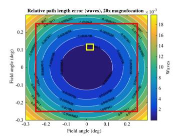
Fig. 9 Relative path length error (waves) for  $20\times$  angular magnification.
