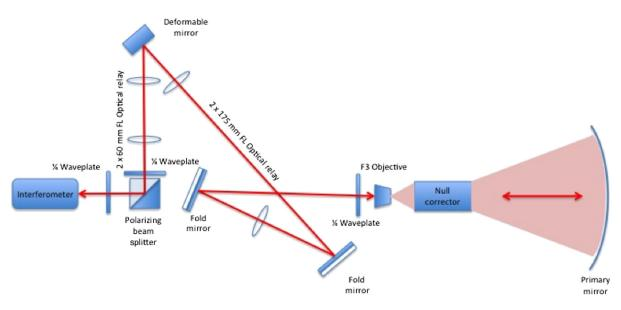
Fig. 13 SMT center of curvature test with deformable mirror and pupil relay optics.
