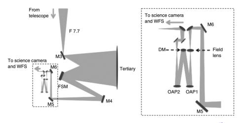
Fig. 8 SMT optical layout with deformable mirror optical relay and pupil size reduced.<sup>15</sup>
