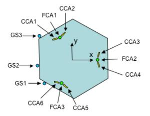
Fig. 4 SMT segment CCA, FCA, and gap sensor (GS) locations.
