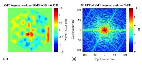
Fig. 6 (a) SMT segment residual OPD in waves and (b) 2-D FFT log plot of SMT residual surface error.<sup>14</sup>
