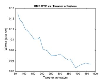
Fig. 11 SMT woofer-tweeter RMS wavefront error versus the number of tweeter actuators.
