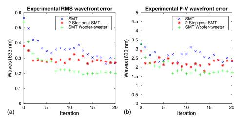
Fig. 15 Experimental SMT and SMT woofer-tweeter wavefront error history using an iterative constrained minimization controller, (a) RMS wavefront error and (b) peak-to-valley wavefront error.
