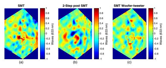
Fig. 16 (a) Experimental SMT wavefront error 0.32 waves RMS, (b) two-step post SMT wavefront error 0.27 waves RMS, (c) and SMT woofer-tweeter wavefront error 0.20 waves RMS.
