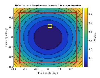
Fig. 10 Relative path length error (waves) for 120× angular magnification.
