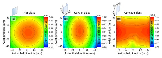
Fig. 2 Relative thickness distribution maps determined by ellipsometry for films on (a) flat, (b) convex, and (c) concave curved glass substrates.
