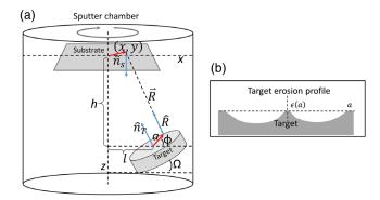
**Fig. 3** A schematic of (a) the sputter chamber geometry where the circular gray arrow indicates that the substrate is rotating during deposition and (b) target erosion profile.
