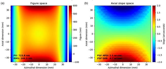
**Fig. 10** (a) Figure and (b) axial slope maps of the deformation caused by nonuniform coating on the concave and convex sides of the optic as calculated using the model presented in Sec. 3. The integrated stress of the coating at the central point is 180 MPa  $\mu$ m on either side, and the integrated stress varies on either side according to the thickness variation presented in Fig. 6. The single-reflection performance of this mirror at 1 keV is 2.6 arc sec HPD.
