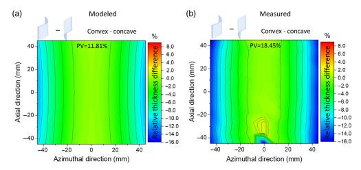
**Fig. 8** The effect of substrate curvature on (a) modeled and (b) measured relative thickness distributions, respectively, examined by subtracting the distributions of a convex substrate from a concave substrate. Note that both figures have the same color scale and PV values are given in this figure.
