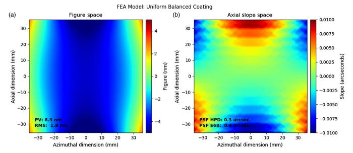
**Fig. 9** (a) Figure and (b) axial slope maps of the deformation caused by the application of uniform, stress balanced thin film coatings to the concave and convex sides of the optic. Shown here is the interior (71.6 mm  $\times$  71.6 mm) area of the mirror. The integrated stress of the coating is 180 MPa  $\mu$ m. The single reflection performance of this optic at 1 keV is 0.3 arc sec HPD, which is consistent with the diffraction limit of an x-ray optic in this geometry.
