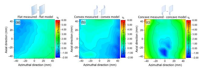
Fig. 7 Relative thickness difference maps showing the modeled relative thickness subtracted from the measured relative thickness for (a) flat, (b) convex, and (c) concave curved substrates. Color scales are the same for all figures.
