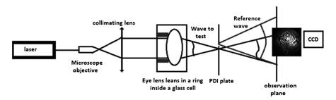
Fig. 1 Point diffraction interferometer setup.
