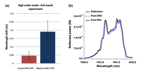
**Fig. 5** (a) Average of the high order wavelength shift after DNA infiltration (red) and after oligonucleotide-functionalized gold nanoparticles (ON-AuNPs) infiltration (blue); a small memory effect decreases the modulation observed for each experiment performed on the same fiber. (b) Spectral measurements after the hybridization process using 100 nM mismatch DNA solution and gold NPs.
