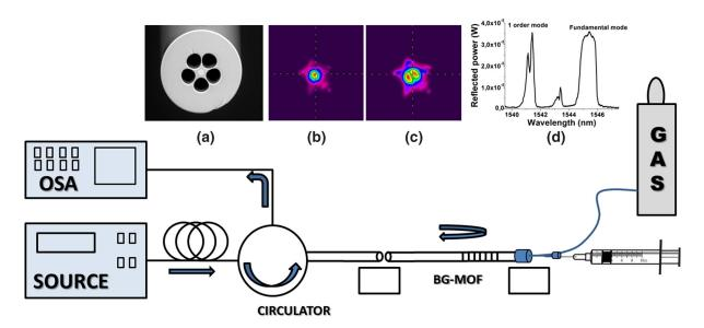
**Fig. 1** The schematic of the optical setup implemented for the experiment is presented. In the top graph, (a) a scanning electron microscope photo of the microstructured optical fiber (MOF) used, with (b) the fundamental and (c) the first order beam profiles. (d) The reflected spectrum of the MOF, revealing a slight birefringence effect.
