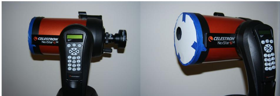
**Fig. 11** Experimental sensor setup consists of a Celestron® NexStar® 6SE 1.5 m focal length telescope with a mask to reduce the aperture to 5 cm, and an Orion® Starshoot™ G3 monochrome camera.
