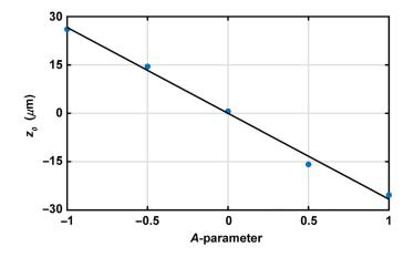
**Fig. 9** PSF *z*-profile peak position ( $z_o$ ) as a function of the *A*-parameter in points. Linear fit in continuous line corresponding to Eq. (5), with a  $R^2 = 0.995$ .
