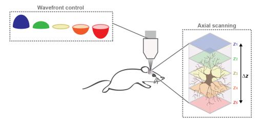
**Fig. 1** A DM is used for manipulating the light beam wavefront reaching the microscope objective entrance pupil and consequently causing different axial displacements of the beam focus over the specimen. This cartoon shows an example of an astrocyte imaged at five different depths.
