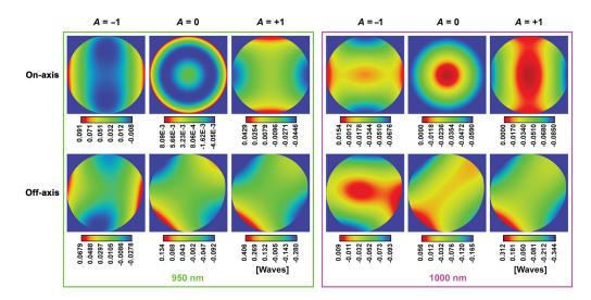
Fig. 7 WFE map across the pupil for six different configurations and two illumination wavelengths (950 and 1000 nm). WFE map units in waves.
