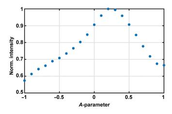
**Fig. 10** Normalized average intensity over the FOV as a function of the DM curvature (given by the *A*-parameter) when imaging a uniform fluorescence slide.
