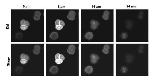
**Fig. 11** Pollen grains imaged at 1040 nm. 2P images acquired at four depths, using the DM (first row), and the objective linear stage (second row). FOV =  $104 \ \mu m \times 104 \ \mu m$ .
