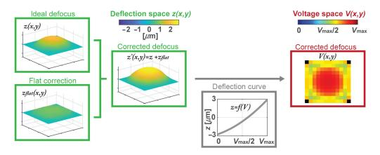
**Fig. 2** Flowchart describing the process from the ideal defocus deflection distribution to the voltage map sent to the DM, in which we consider the flat correction needed to flatten the intrinsic DM bow and the DM deflection curve.
