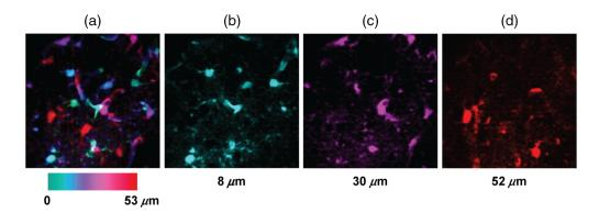
**Fig. 13** *In vivo* brain imaging of astrocytes illuminated at 1020 nm. 2P *z*-stack acquired using the DM to change the depth in steps of  $\delta z = 0.3 \ \mu$ m. (a) Maximum intensity *z*-projection color-coded by depth. FOV = 306  $\mu$ m × 306  $\mu$ m × 53  $\mu$ m. Single frames taken at depths of (b) 8, (c) 30, and, (d) 52  $\mu$ m.
