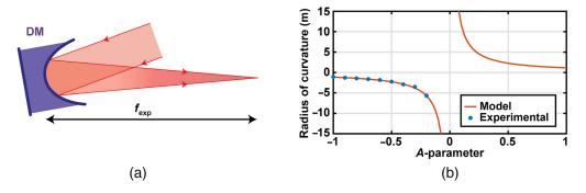
**Fig. 3** (a) A collimated light beam is focused at a distance  $f_{exp}$  by the DM with a concave shape. (b) Experimental and theoretical DM radius of curvature as a function of the *A*-parameter.
