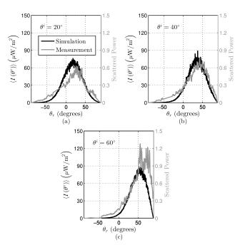
**Fig. 6** Average scattered irradiance and measured scattered power versus observation angle  $\theta^r$  for the LabSphere Infragold sample. The average scattered irradiance was calculated by averaging the scattered irradiance, predicted using the MoM, over 400 independent surface realizations generated using the LabSphere Infragold's measured roughness statistics. The scattered power measurements were taken using the CASI. The angles of incidence are (a) 20 deg, (b) 40 deg, and (c) 60 deg.
