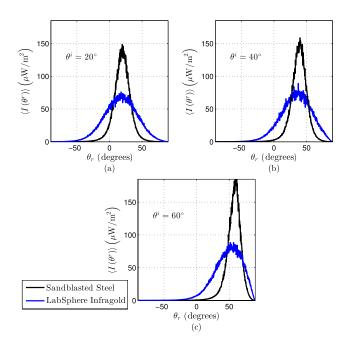
Fig. 9 Average scattered irradiances for LabSphere Infragold and sandblasted steel. Angles of incidence are (a) 20 deg, (b) 40 deg, and (c) 60 deg.
