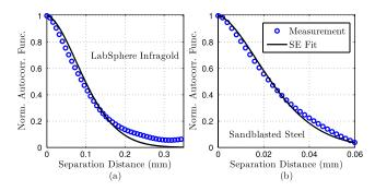
Fig. 3 SE nonlinear least-squares fits to measured autocorrelation data. (a) LabSphere Infragold normalized autocorrelation function fit; and (b) sandblasted steel normalized autocorrelation function fit.
