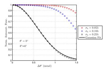
**Fig. 8** Normalized autocorrelation functions of the far-zone scatteredfield at normal incidence and normal observation for simulated rough Gaussian surfaces as surface roughness is varied. For  $\sigma_h = 0.05\lambda$ and  $\sigma_h = 0.1\lambda$ , the normalized autocorrelation functions are non-Gaussian and approach an asymptotic value for large separation angles. The normalized autocorrelation function is very nearly Gaussian for  $\sigma_h = 0.25\lambda$ .
