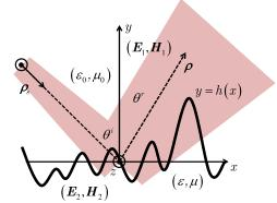
**Fig. 1** Scattering geometry of a one-dimensional, rough impedance surface (i.e., the surface and source excitation are invariant in the *z* direction). The medium below the rough interface has a permittivity of  $\varepsilon$  and a permeability of  $\mu$ . The medium above the rough interface is vacuum.
