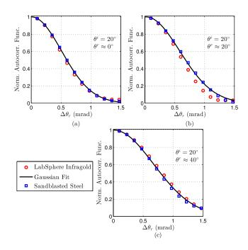
**Fig. 10** Normalized autocorrelation functions of the far-zone scattered field of LabSphere Infragold and sandblasted steel in different observation directions. In all the plots, the angle of incidence is 20 deg. The observation directions are (a) 0 deg (normal), (b) 20 deg (specular), and (c) 40 deg. The normalized autocorrelation functions are nearly Gaussian, with very similar angular widths for both samples. Note that the angular widths are different depending on the observation direction.
