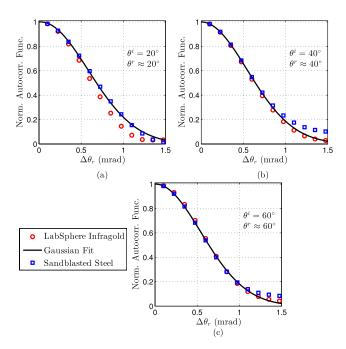
**Fig. 11** Normalized autocorrelation functions of the far-zone scattered field of LabSphere Infragold and sandblasted steel when observation is in the specular direction. The angles of incidence are (a) 20 deg, (b) 40 deg, and (c) 60 deg. The angular widths for all three cases are nearly identical.
