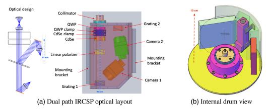
**Fig. 3** (a) Optical layout of dual-path IRCSP and (b) inside of the instrument with the lid removed. The maximum allowable envelope for the IRCSP subsystem is 120 ml or 0.12 U and is shown as the transparent green box in (b). This volume constraint for the IRCSP limited the detector choice to uncooled microbolometers.
