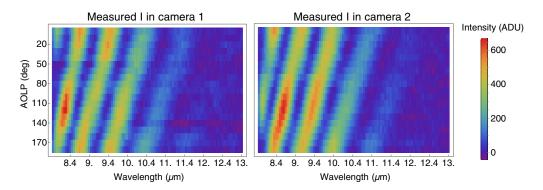
**Fig. 8** The estimated intensity  $\hat{l}_c$  as a function of AOLP and wavelength for DOLP = 1 calculated using the spectral assignment procedure discussed in Sec. 4.1.3.
