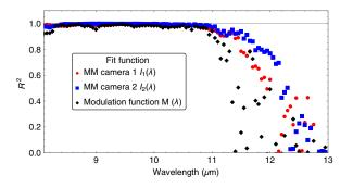
**Fig. 14** Comparison of the coefficient of determination ( $R^2$ ) for the fit of the calibration data to the Mueller matrix model for  $I_c(\lambda)$  and the modulation function  $M(\lambda)$ .
