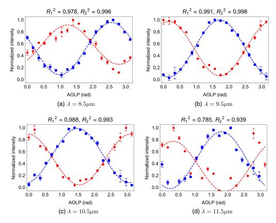
**Fig. 7** Fit of normalized intensity in camera 1 (red) and camera 2 (blue) to Mueller matrix model in Eq. (6) for  $\lambda = 8.5$ , 9.5, 10.5, and 11.5  $\mu$ m.  $R^2$  [Eq. (12)] values for each fit are shown above figures. Modulation is better in the transmitted path, as seen by the higher camera 2  $R^2$  as compared to camera 1. A significant reduction in  $R^2$  values for both cameras is observed at the highest wavelength.
