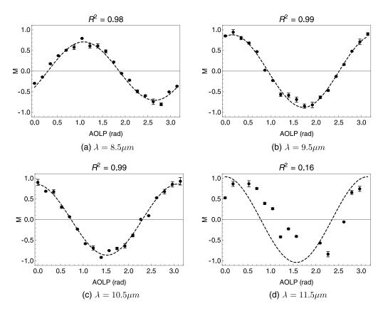
**Fig. 11** Fit of measured modulation function to Eq. (9) for  $\lambda = 8.5$ , 9.5, 10.5, and 11.5  $\mu$ m.  $R^2$  values [Eq. (12)] for each fit are shown above figures. As with the Mueller matrix model fits (Fig. 7), there is a significant reduction in  $R^2$  past 11  $\mu$ m.
