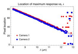
Fig. 4 The pixel location of the diffracted order in each path as a function of wavelength. A linear fit is applied to the pixel location of the maximum intensity calculated during calibration.
