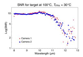
Fig. 9 The calculated log (SNR) at room temperature for cameras in path 1 (reflection) and path 2 (transmission) to unpolarized light calculated from the data in Fig. 6. SNR declines abruptly past 11  $\mu$ m.
