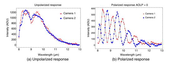
**Fig. 6** Measured response  $\hat{I}_c$  in camera 1 (reflection, red) and camera 2 (transmission, blue) to: (a) unpolarized light and (b) polarized light with DOLP = 1 and AOLP = 0 deg. The response is reported as the analog digital count (ADU). Departure from equal cameras 1 and 2 measurements for unpolarized illumination indicates polarization-dependent efficiency in the DG following the linear polarizer.
