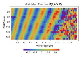
**Fig. 10** The modulation function  $\hat{M}$  [Eq. (9)] computed from fully polarized narrowband calibration measurements as a function of AOLP and wavelength. The modulation function is degraded at wavelengths higher than 11  $\mu$ m due to the camera SNR reported in Fig. 9.
