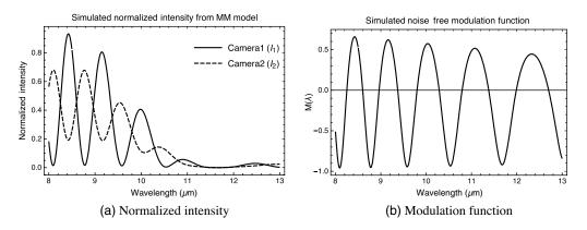
**Fig. 2** Simulated noise-free modulation function: (a) the intensity in paths 1 and 2 and (b) the modulation function. The frequency of modulation is proportional to  $1/\lambda$  due to the dispersion of CdSe. Reduced contrast from the linear polarizer in reflection causes the modulation function to be reduced.
