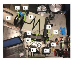
**Fig. 5** Layout of the monochromator testbed at GSFC. The components are 1. black body source, 2. optical chopper, 3. monochromator input slit, 4. monochromator, 5. output slit, 6. spectral filter wheel, 7. off-axis parabolic mirror, 8. fold mirror, 9. reference detector, 10. linear polarizer on rotating mount, and 11. IRCSP.
