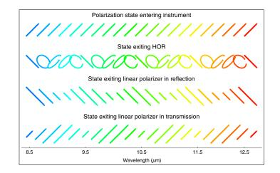
**Fig. 1** The transformation of broadband linearly polarized light with constant DOLP and AOLP as propagated through the IRCSP Mueller matrix model. The polarization is altered as a function of wavelength as it passes through the QWR and HOR. Following the HOR, the beam is split and modulated by a linear polarizer in reflection and transmission.
