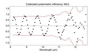
**Fig. 13** Polarimetric efficiency of the system  $\hat{W}(\lambda)$  for narrowband light in red plotted over the measured modulation for AOLP = 0. Efficiency is greater than 0.8 from 8 to 11  $\mu$ m.
