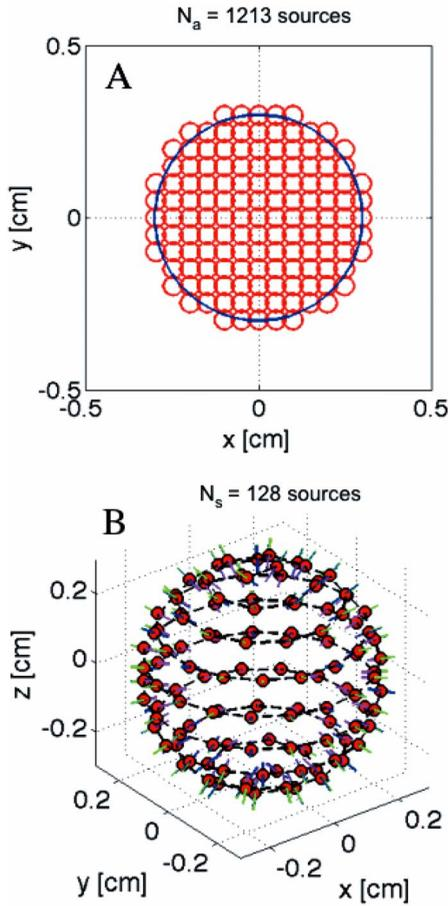
**Fig. 8** The virtual sources for perturbation by an object. (a) Subvolumes within an object, accounting for object absorption and scattering-enhanced absorption. (b) Surface sources on the object's surface, creating a dipole oriented along the gradient of fluence rate.
