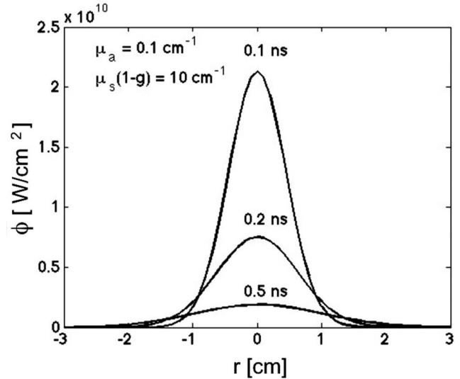
Fig. 3 Time-resolved diffusion of light from an impulse of light,  $Q = 1$  J, delivered as a point source at  $r=0$ ,  $t=0$ . The time-resolved fluence rate  $\phi(r,t)$  is shown at  $t=0.1$ ,  $0.2$ , and  $0.5$  ns.
