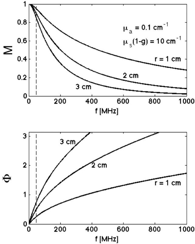
**Fig. 6** Modulation ( $M$ ) and phase ( $\Phi$ ) versus frequency of modulation, observed at  $r=1, 2,$  and  $3$  cm from source. The source modulation and tissue properties are the same as in Fig. 5.
