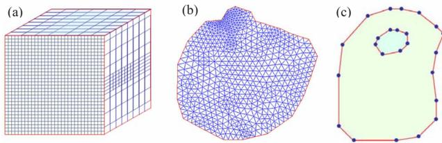
**Fig. 12** Example meshes are shown for (a) finite difference solver in Cartesian coordinates with adaptive mesh refinement in each of the  $x, y, z$  directions; (b) finite element solver using triangular elements in two dimensions or tetrahedral elements in three dimensions; and (c) a boundary element solver where the mesh is just composed of nodes at the boundaries outlining homogeneous regions.
