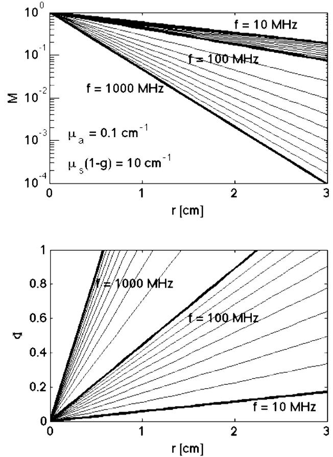
**Fig. 5** Modulation ( $M$  [dimensionless]) and phase ( $\Phi$  [radians]) versus distance ( $r$  [cm]) of observation point from source, for various frequencies ( $f$  [Hz]) of full source modulation,  $M_o=1$ . Optical properties of medium are absorption  $\mu_a=0.1 \text{ cm}^{-1}$ , and reduced scattering  $\mu_s(1-g)=10 \text{ cm}^{-1}$ .
