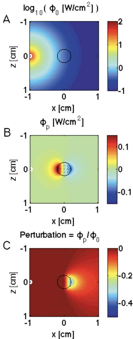
**Fig. 10** An object with increase scattering ( $\mu_{s0}=0.1 \text{ cm}^{-1}$ ,  $\mu_{s0'}=10 \text{ cm}^{-1}$ ,  $\Delta\mu_a=0$ ,  $\Delta\mu_s'=10 \text{ cm}^{-1}$ ). (a), (b), and (c) are the same as in Fig. 9. The object asserts a dipole pattern of perturbation, in which light is scattered upstream toward the source, and a shadow is cast downstream. However, the perturbation has little effect upstream toward the source of light.
