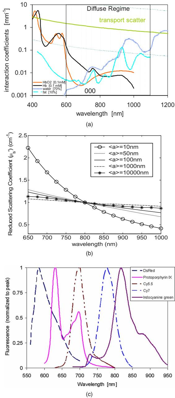
**Fig. 14** (a) The absorption spectra of the major chromophores in tissue are shown along with a typical reduced scattering spectra. The changes to the reduced scattering spectra with Mie-like scatterer size change are shown in (b).<sup>59</sup> The luminescence spectra for several known endogenous emitters is shown in (c).
