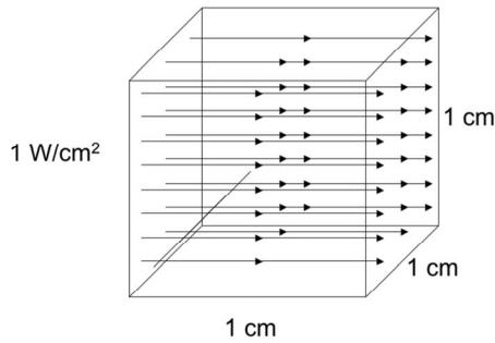
**Fig. 2** The concentration of photons in a cube of water irradiated with  $1 \text{ W/cm}^2$  is  $0.18 \text{ pM}$ .
