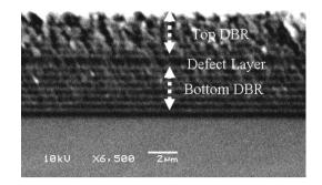
**Fig. 3** Cross-sectional scanning electron micrograph (SEM) of the fabricated multilayer stack obtained by cleaving through one of the diffractive levels. The layered structure consisting of nitride (lighter regions) and oxide (darker regions) layers with an oxide defect layer is clearly seen in the micrograph.
