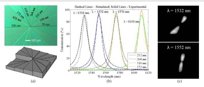
**Fig. 4** (a) Optical microscope image of the charge 2 vortex elements and schematic. (b) Simulated (dotted lines) and experimental transmission spectra. (c) Images of the spatial transmission through the vortex element at 1532 nm and 1553 nm. The vortex element was illuminated using a beam of diameter 3 mm.
