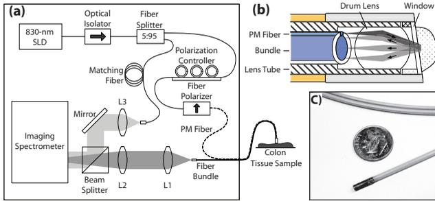
**Fig. 1** a/LCI system diagram. (a) System illustration, (b) probe tip assembly illustration showing delivered (dark gray) and scattered (light gray) light, and (c) photograph of the endoscopic probe pictured next to a U.S. dime for scale. Illustration adapted from Zhu et al. (Ref. 22).
