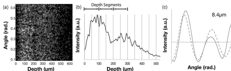
**Fig. 2** Typical a/LCI data. (a) Angle-resolved depth scan of light scattered from tissue. Lighter shades of gray indicate an increased amount of scattered light. (b) A-scan indicating depth increments used for processing. Fifty micrometer segments of the tissue used for processing are indicated. (c) Example angular scan pictured (solid line) with best-fit Mie theory solution (dashed line) and size indicated.
