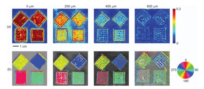
**Fig. 5** Images of the (a) SOI and (b) structure orientation from an experiment in which a layer of highly scattering material was put on top of the fibrous samples. The top layer was varied in thickness from 0 to 600  $\mu$ m.
