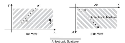
**Fig. 1** Schematic of the experimental geometry. Gray rectangles represent cylindrical light scattering structures in a turbid medium. Left: top view of the medium where  $\varphi$  is the angle in the *x*-*y* plane between the wave number **q** of the sinusoidal illumination pattern, and the projection of the cylindrical structures onto the *x*-*y* plane. Right: side view of the medium where  $\theta$  is the angle between the surface and the cylinder direction.
