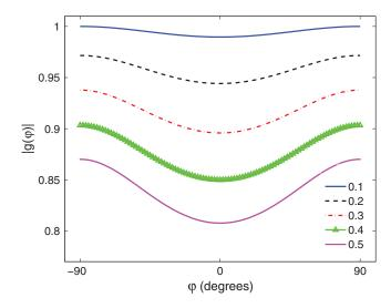
**Fig. 2** Plot of the calculated amplitude of remitted light as a function of the angle  $\varphi$  between the wave number of the projected sinusoidal pattern, and the direction of the cylindrical scattering structures. The amplitudes due to 5 projection frequencies ranging from 0.1 to 0.5 mm<sup>-1</sup> are shown. The minimum occurs when the wave number is aligned with the scattering structures. Higher frequencies are more sensitive to anisotropy, but have smaller average amplitude.
