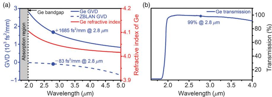
**Fig. 1** (a) GVD and refractive-index curves of Ge and GVD curve of ZBLAN fiber. Sellmeier equations of Ge and ZBLAN are used from Refs. 18 and 19. (b) Transmission curve of 2-cm-long anti-reflection-coated Ge rod measured using a Fourier-transform spectrometer.
