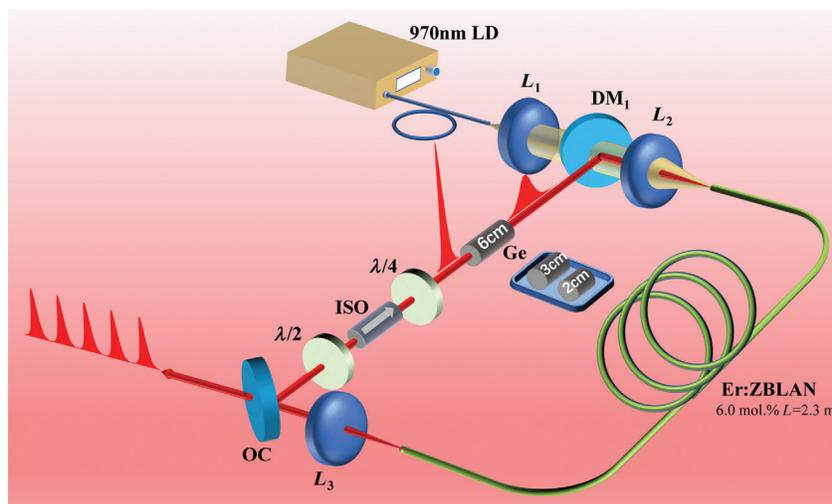
**Fig. 2** Schematic of the breathing-pulse mode-locked Er:ZBLAN fiber laser. LD, laser diode; DM, dichroic mirror; OC, output coupler with a transmission of 40%; ISO, optical isolator;  $\lambda/2$ , half-wave plate;  $\lambda/4$ , quarter-wave plate; and Ge, germanium rod.
