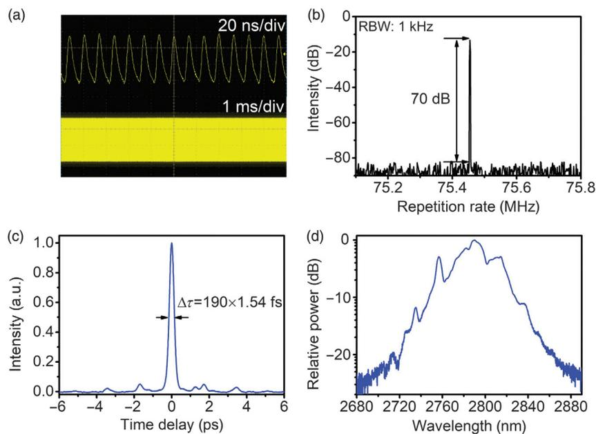
**Fig. 3** Soliton mode-locked Er:ZBLAN fiber laser: (a) pulse trains in nanosecond and millisecond time scales, respectively; (b) radiofrequency spectrum; (c) measured intensity autocorrelation trace; and (d) mode-locked pulse spectrum.
