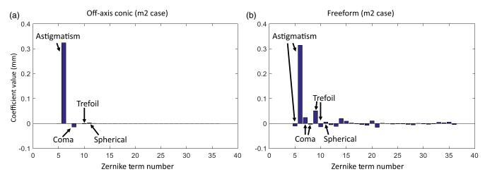
Fig. 4 Surface decomposition of a powered surface in a K-mirror system whose surface profile is specified using (a) the off-axis conic parameters or (b) Zernike coefficients in standard ordering. The surface decomposition was performed with 36 Zernike terms in standard ordering over the circular aperture of the mirror.
