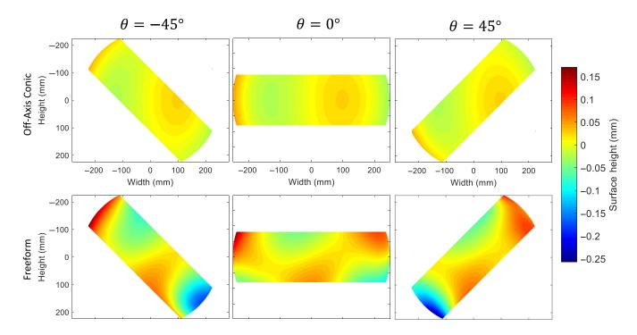
**Fig. 7** Subaperture samples of the powered mirror (as shown in Fig 6) in the K-mirror instrument, where each configuration is a rotation of the K-mirror about its axis by 45 deg. The freeform surface is able to generate the local surface control that the design requires while the off-axis conic is stuck with an entangled ratio of terms that are generated by obtaining the correct amount of astigmatism.
