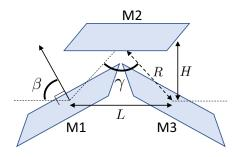
**Fig. 2** Diagram of the parameters used to define the layout of a K-mirror image rotator, where *L* and *H* could be specified by packing restrictions, which determine the required folding angle  $\gamma$ , spacing between mirrors *R*, and angle of incidence  $\beta$ . M1, M2, and M3 are the labels for the mirrors in the system, where light travels from M1 to M2 and finally to M3.
