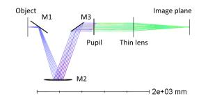
**Fig. 5** Optical layout of the K-mirror system used to perform the design comparison experiments. Note that this is one configuration of the K-mirror, where to produce the image derotation, the system (M1 to M3) rotates about the optical axis (horizontal), causing the light from the various fields to move on the optical surfaces.
