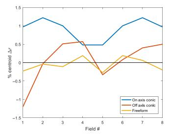
**Fig. 9** Percent radial difference in centroid location between the ideal and the as-designed coordinates for eight field points in the instrument FOV averaged across the 5 K-mirror configurations ( $\theta = -45$  deg, -22.5 deg, 0 deg, 22.5 deg, and 45 deg).
