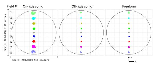
**Fig. 8** Comparison between the distortion correction achieved between the on-axis conic, off-axis conic, and freeform designs. The image planes for each design are shown with the focused spots from each K-mirror position on top of one another. Distortion is defined as the shift in focus location with respect to the ideal focus, computed using a thin lens model. The distortion of each point in the FOV is computed in all three designs, as given in Fig. 9.
