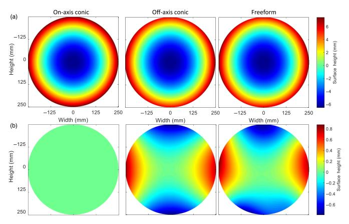
**Fig. 6** Surface sag maps of M2 in the K-mirror systems. (a) The full surface sag and (b) the Zernike power term (Z4) removed to highlight the local surface control achieved by using a freeform surface specification. The local control gained in the freeform surface means that configuration-dependent aberrations can be better corrected.
