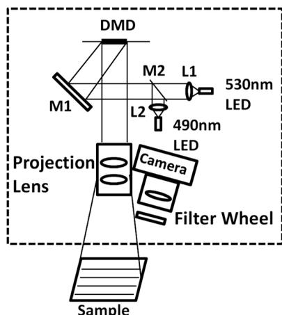
**Fig. 1** Optical layout of ACF imaging system. Patterns are generated on the digital micromirror device, illuminated by LEDs, and projected by the projection lens to the sample. Filter wheel is used to select the wavelength and the imaging field is captured by a CCD camera.
