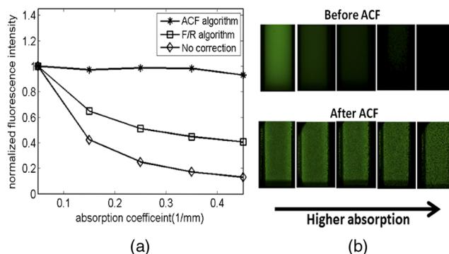
**Fig. 2** (a) Normalized fluorescence intensity of *in vitro* tissue phantom with ACF correction,  $F/R$  correction, and no correction for phantom set with  $\mu'_s = 1.0 \text{ mm}^{-1}$ . (b) The 2-D fluorescence image before and after the ACF correction.
