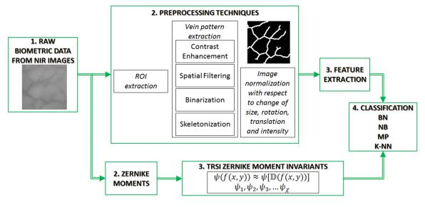
**Fig. 1** Flowchart of a hand vein recognition system: traditional approach (top stream) and the proposed approach (bottom stream). As the sensed image  $\mathbb{D}(f(x, y))$  is a degraded version of the original scene f(x, y), then the invariant vector  $\psi_1, \psi_2, \ldots, \psi_{\chi}$  satisfies that  $|\psi(f) - \psi(\mathbb{D}(f(x, y)))| \approx 0$ .
