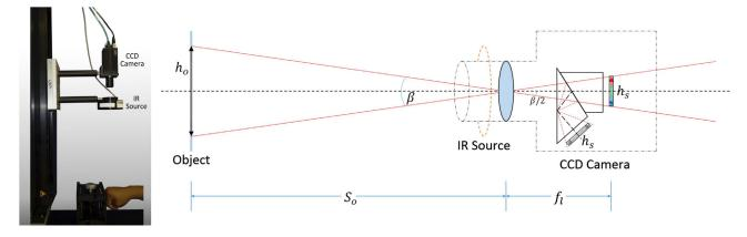
Fig. 2 Infrared hand vein acquisition system.
