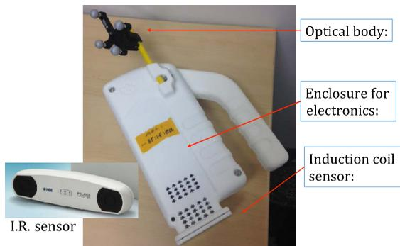
Fig. 1 IR sensor and optical body mounted on attached mast.
