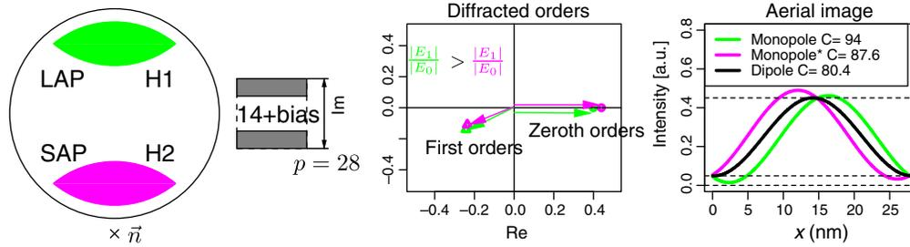
**Fig. 11** Dipole illumination on the left for a 28-nm pitch L/S grating, phasor diagram, and resulting aerial images for monopoles and dipole. In the case of horizontal patterning in EUV, we have different images for the small angle pole (magenta) and the large angle pole (green). Reprinted from an article of Burkhardt.<sup>100</sup>
