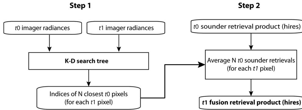
**Fig. 1** Schematic of the LEO sounder to GEO imager temporal resolution fusion approach. All input and output data are at high spatial resolution (hires).
