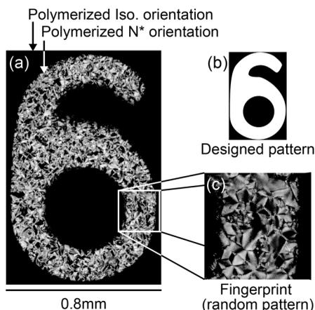
**Fig. 1** Schematic of the proposed optical security device, providing both the designed pattern and the fingerprint: (a) polarizing microphotograph of the device; (b) the designed pattern stored in this device; and (c) the fingerprint or unique identification pattern.
