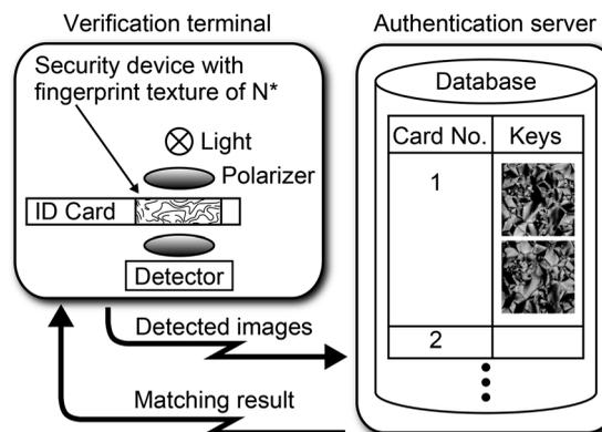
**Fig. 4** Schematic diagram of a basic security system using the proposed devices.
