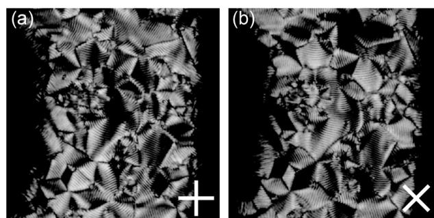
**Fig. 3** Polarizing microphotographs taken in the same area of the same device under two different crossed polarizer configurations. The crosses represent the directions of the crossed polarizers.
