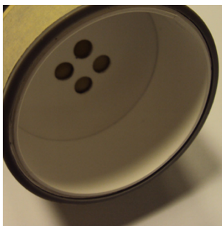
Fig. 1 Prototyped cylindrical mixing chamber constructed out of MCPET including four uniform Lambertian light sources created by partially covering a remote phosphor LED module with an MCPET baseplate.
