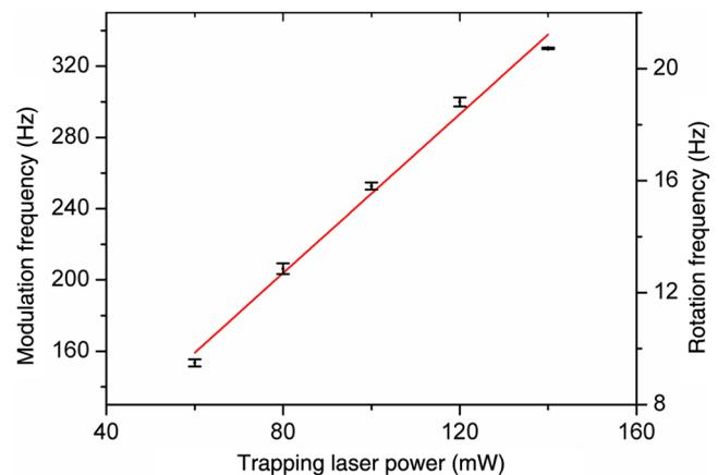
**Fig. 6** Beat frequency and calculated rotation frequency versus the trapping laser power for probe beam of  $l = \pm 8$ . The error bars denote the FWHMs of the spectral peak. The red solid line represents the linear fitting result.
