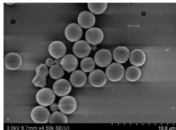
**Fig. 4** SEM image of the silk fibroin regulated vaterite microspheres.
