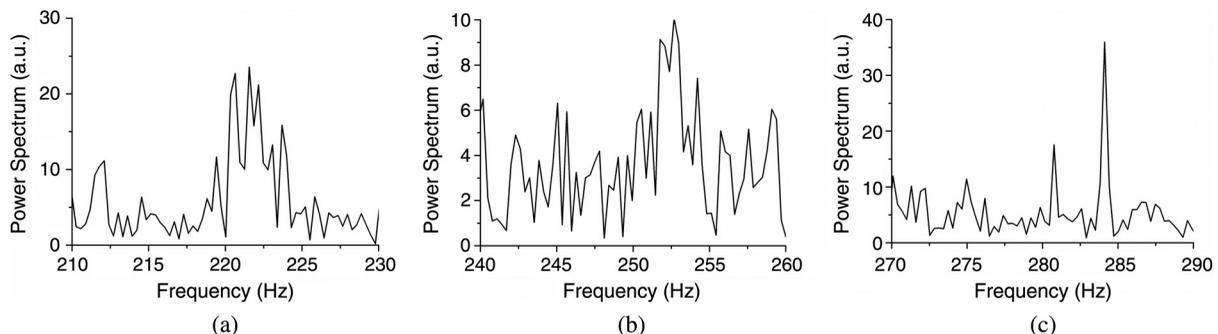
**Fig. 5** Power spectra for probe beams consisting two LG lights of (a)  $l = \pm 7$ , (b)  $l = \pm 8$ , and (c)  $l = \pm 9$ . The corresponding beat frequencies are  $221.9 \pm 1.7$  Hz,  $252.5 \pm 0.8$  Hz, and  $284.1 \pm 0.2$  Hz (measured as FWHM).
