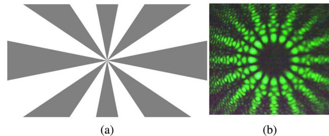
**Fig. 3** (a) Phase profile of LG  $\pm 8$  modes and (b) corresponding far-field intensity profile.
