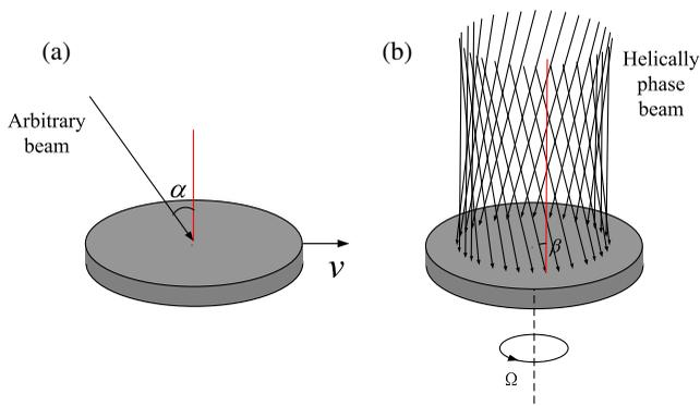
**Fig. 1** (a) Linear Doppler effect and (b) rotational Doppler effect.
