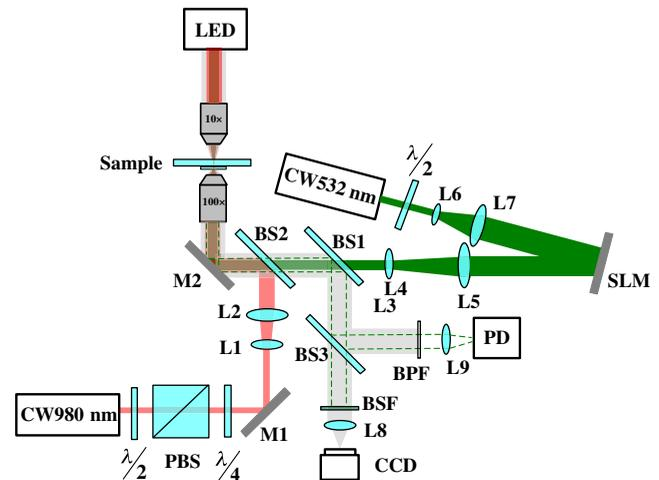
**Fig. 2** The experimental setup used for the rotational Doppler effect. Labels denote the continuous wave (CW), half-wave plate ( $\lambda/2$ ), polarizing beam splitter (PBS), quarter-wave plate ( $\lambda/4$ ), mirror (M), lenses (L), beam splitter (BS), SLM, bandpass filter (BPF), bandstop filter (BSF), and photodiodes (PD)
