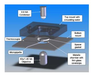
**Fig. 3** Custom micromanipulation chamber comprised of mounting plate, silicone spacers, metallic chamber with a side aperture, thermocouple for temperature monitoring, micropipette for micromanipulation, and the water circulation chamber.
