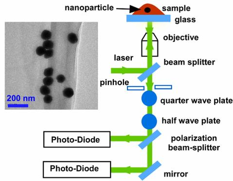
Fig. 1. Schematic diagram of the measurement setup. Inset shows TEM image of gold nanoparticles.
