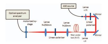
Fig. 1 Experimental S<sup>2</sup> imaging setup.
