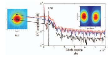
**Fig. 5** Example of the S<sup>2</sup> imaging measurement on a 1-m length polarization maintaining LMA step-index fiber with 0.06NA and 15- $\mu$ m mode field diameter: (a) Typical intensity profile and (b) example Fourier transforms at three different scan points, shown with dark dots on (a) and reconstructed intensity image of the LP11 mode, HOM suppression -24.1 dB.
