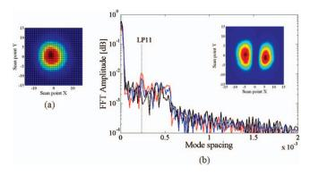
**Fig. 8** Example of the S<sup>2</sup> imaging on a 2.2-m DC-200/40-PZ-Yb-03 having 29- $\mu$ m mode field diameter and NA of 0.03: (a) Example intensity profile and (b) example Fourier transforms at three different points at the beam, selected as in Fig. 5, and the reconstructed intensity image of LP11 mode, HOM suppression – 24.7 dB.
