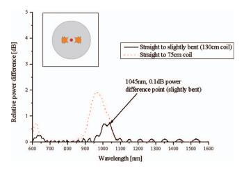
**Fig. 3** Transmission measurement of a polarization maintaining stepindex LMA fiber with a 0.06 NA and 15  $\mu$ m mode field diameter, showing the wavelength where the HOM content is suppressed by -20 dB. The fiber design is illustrated in the inset.
