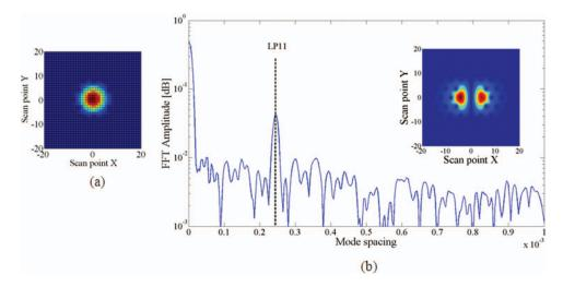
**Fig. 2** (a) Simulated intensity profile of the fundamental mode and the 100 times weaker higher order mode after traveling through a standard PCF of 40- $\mu$ m core diameter. (b) Example Fourier transform, shown as a function of mode spacing, which is defined by the effective index difference between the interfering modes, and reconstructed intensity profile of the -20-dB suppressed LP11 mode.
