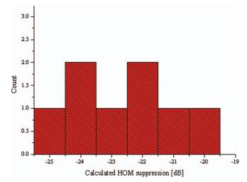
Fig. 6 Histogram of the measured HOM suppressions obtained with the S<sup>2</sup> imaging, while offsetting the input beam and varying the width of the Fourier integration window when calculating the HOM suppression. The average HOM suppression is  $-22.5 \pm 3$  dB.
