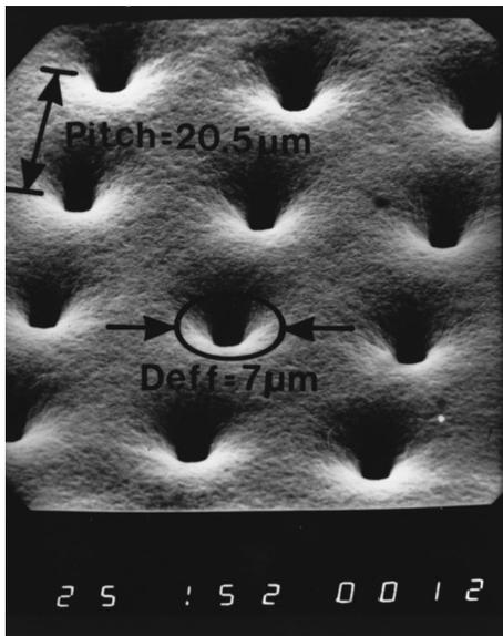
**Fig. 1** A section of the cell carrier.
