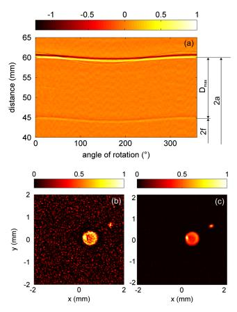
**Fig. 3** (a) Recorded raw data showing the difference of the SNR of signals recorded with and without the influence of the acoustic mirror. (b) Image using the direct wave data. (c) Section image using the focused wave.
