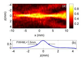
**Fig. 2** (a) Dependence of the measured signal amplitude on the source position. The center of the image at x = 0 marks the position of the focal line F2. (b) Averaged *z* profile indicating the resolution between neighboring sections.
