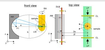
Fig. 1 Front and top view of the optical section imaging setup.
