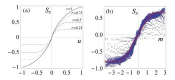
**Fig. 2** Sensor calibration: (a) expected response normalized using an incoherent disc source for different radii; (b) plot of the signals (blue dots) versus slope and the fit (red curve) used to linearize the sensor response.
