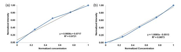
Fig. 9 (a) Fluorescent target emission intensity recorded with a spectrometer as a function of dye concentration. (b) Fluorescent target SFE image intensity as a function of dye concentration.
