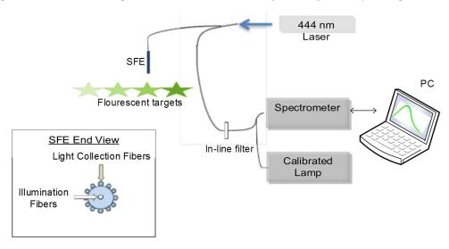
Fig. 2 Schematic diagram of the experimental setup to quantify targets' fluorescence.
