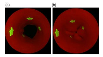
**Fig. 11** SFE fluorescence and red reflectance dual-modal imaging of the phantom. Dual-modal SFE imaging of the phantom with four 100  $\mu$ mol/L fluorescent targets. Left: sphincter open. Right: sphincter closed.
