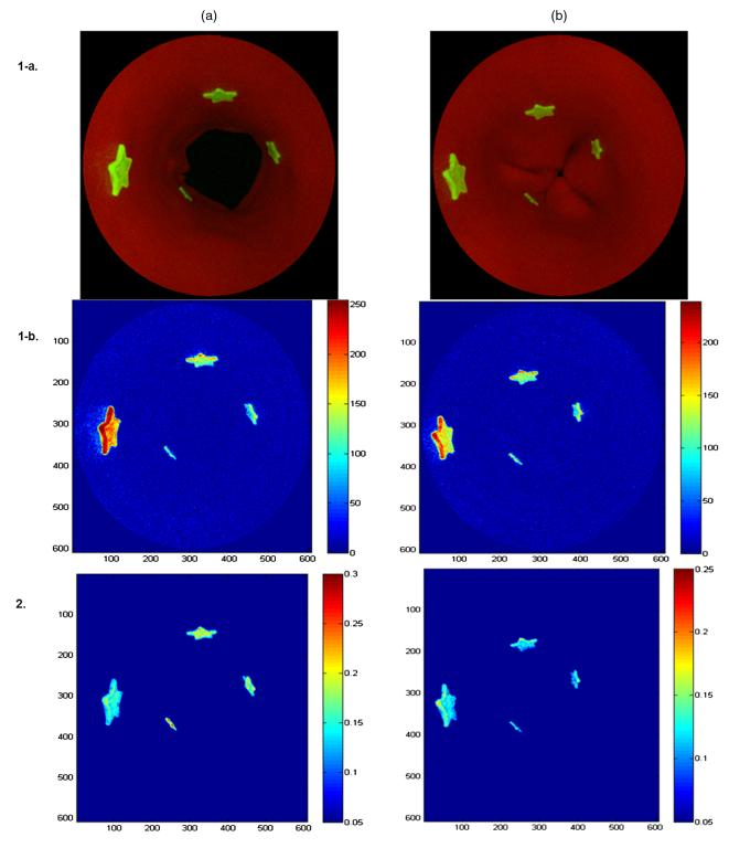
**Fig. 12** Phantom application: the SFE distance compensation (DC) algorithm development. (a) Sphincter open mode; (b) sphincter closed mode; (1-a) before DC SFE dual-mode (reflectance-fluorescence) image; (1-b) before DC colormap of the fluorescence image from (1-a); (2) After DC colormap of the fluorescence image from (1-a).
