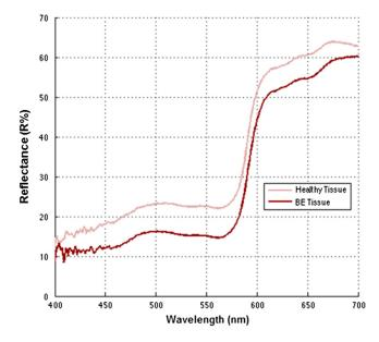
Fig. 6 Diffuse spectra reflectance of simulated healthy esophagus and BE tissue from the phantom.
