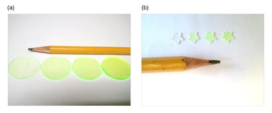
Fig. 8 Photo representations of dye-in-polymer. (a) ~750 µm thin disks, (b) die-cut distinctive star shaped targets.
