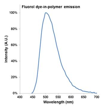
**Fig. 7** Fluorol dye-in-polymer emission spectra under 444 nm laser excitation, measured by a calibrated spectrometer.
