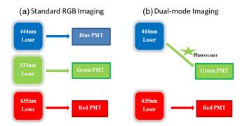
**Fig. 3** (a) Standard SFE RGB imaging; (b) SFE dual mode imaging, with the 532 nm blue photomultiplier tube (PMT) channel inactive.
