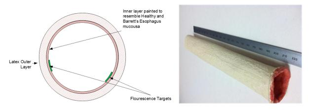
Fig. 1 (a) A cross-sectional graph illustrating the phantom design. (b) An overview of the resultant phantom.
