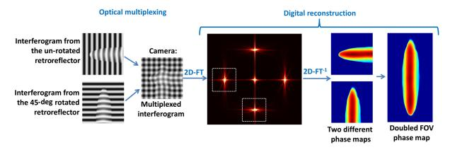
**Fig. 2** Digital processing of the multiplexed interferogram into two different quantitative phase maps, which can be stitched together. 2D-FT, two-dimensional Fourier transform; 2D-FT<sup>-1</sup>, two-dimensional inverse Fourier transform.
