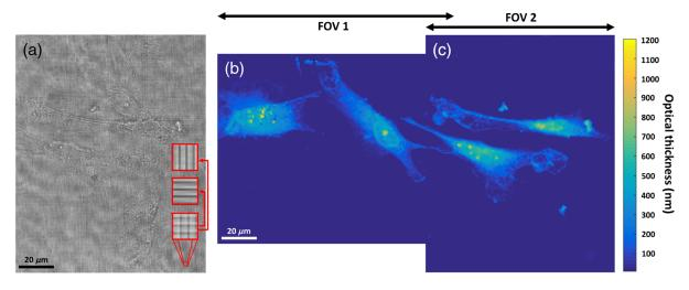
**Fig. 5** Melanoma cancer cells, as captured by the broadband off-axis interferometer, enhanced with the proposed FOV-doubling module. (a) The multiplexed interferogram captured by the digital camera. In red boxes—magnified image of the multiplexed interference fringes, and the two off-axis interference fringe patterns composing it. (c) The stitched quantitative phase map.
