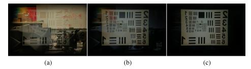
**Fig. 8** Demonstration of the tunable image contrast with different voltage applied to the liquid crystal glass: (a) 0 V, (b) 2.5 V, and (c) 5 V.
