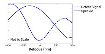
Fig. 3 Schematic diagram of the defect signal and the speckle noise through-focus behavior. Defect type: dense line intrusion defect with a size about  $26 \times 26$  nm<sup>2</sup> on the mask.
