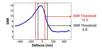
Fig. 8 Defect SNR through-focus behavior for isoline extrusion critical defect. Pixel size:  $30 \times 30$  nm<sup>2</sup>. Photon density: 50 photons/nm<sup>2</sup>. Defocus range:  $\pm 500$  nm. Black box: defocus range: -100 to +100 nm. Red box: -150 to +50 nm. The best focus position is defined as the position with minimum speckle contrast, as shown in Fig. 3.
