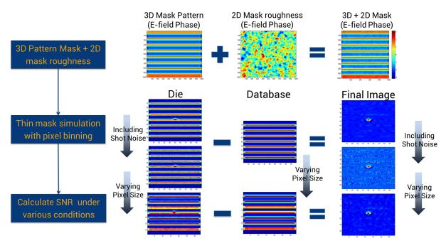
Fig. 2 Schematic diagram of the defect SNR calculation process flow.
