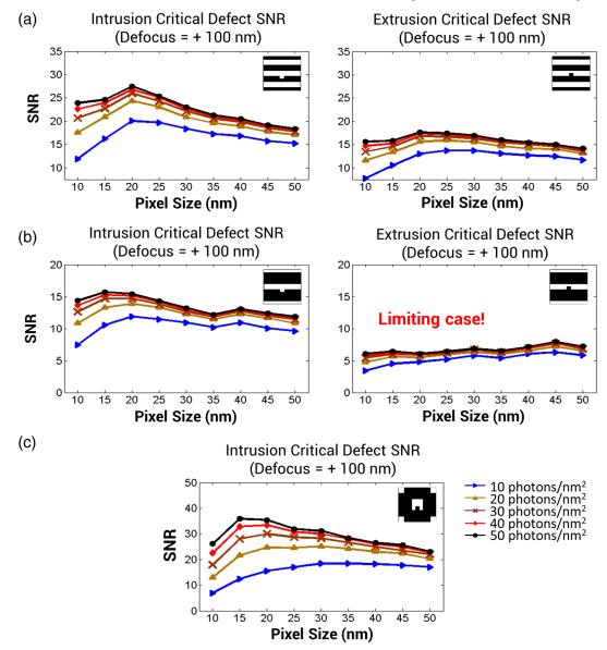
**Fig. 7** Critical defect SNR at defocus position = +100 nm for various patterns: (a) dense line, (b) isoline, and (c) dense contact. Legends in (c) indicate the photon density level for each curve, ranging from 10 to 50 photons/nm<sup>2</sup>. The best focus position is defined as the position with minimum speckle contrast, as shown in Fig. 3.
