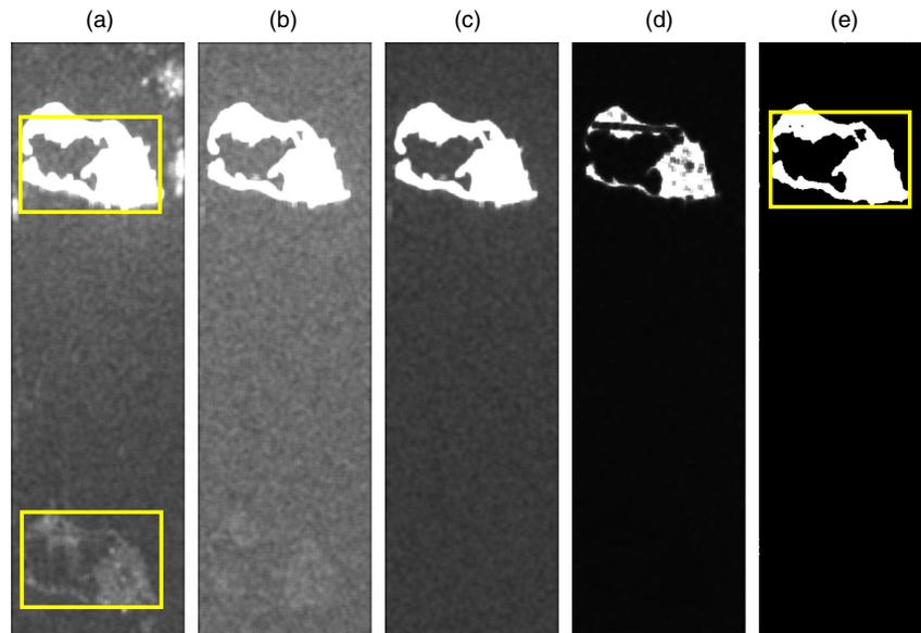
**Fig. 4** An example of SAR azimuth ambiguity removal using RMSRP. The bright target is Dongsha Island in East China Sea. (a)  $|HH|$ , (b)  $|HV|$ , (c)  $|HV + VH|$ , (d) RMSRP, (e) Detection result.
