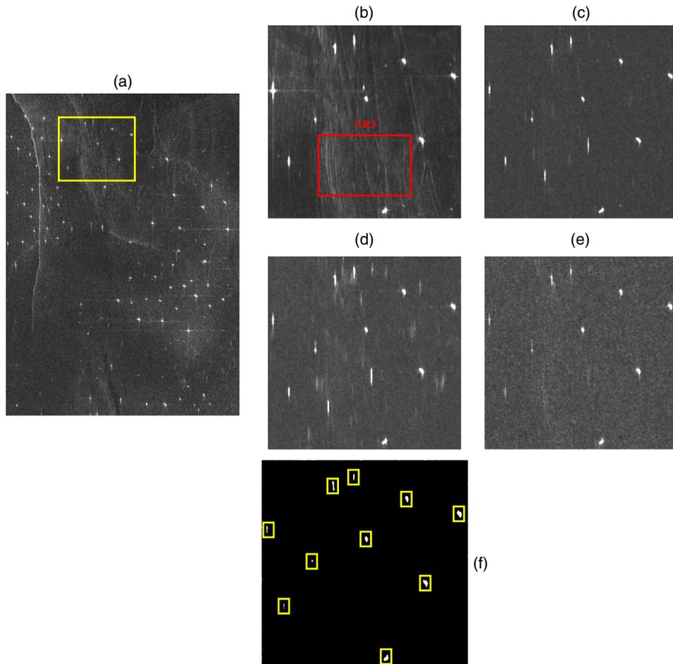
**Fig. 6** Another example of target detection in noise-corrupted SAR image (named RS\_ VI in Table 1). (a) |HH|, (b) |HH|, (c) |HV|, (d) |HV + VH|, (e) RMSRP, (f) Detection result.
