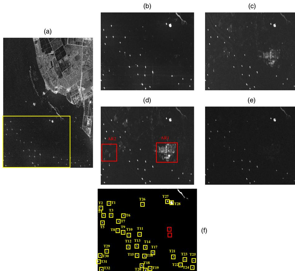
**Fig. 5** An example of target detection in noise-corrupted SAR image (RS\_V in Table 1). (a)  $|HH|$ , (b)  $|HH|$ , (c)  $|HV|$ , (d)  $|HV + VH|$ , (e) RMSRP, (f) Detection result.
