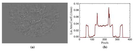
Fig. 4 (a) Difference image between Fig. 3(b) and 3(d) in the display window of [-0.02.0.1]mm<sup>-1</sup>. (b) Profiles across the lines shown in the images of Fig. 3(b) and 3(d). The solid line represents the profile of Fig. 3(b) and the dotted line that of Fig. 3(d).
