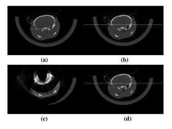
**Fig. 3** The reconstructed images corresponding to (a) a full data sampling case, (b) an existing sparse-view case, (c) a statically collimated case, and (d) a sinusoidally collimated case.
