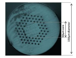
Fig. 1 Microscope image of end face of multimode mPOF.
