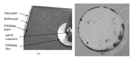
Fig. 3 Fiber polishing process and mPOF in ferrule connector after polishing.
