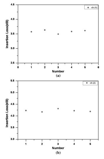
Fig. 9 Insertion loss changes after 5 h at port 1 (a) and port 2 (b).
