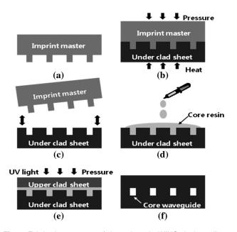
**Fig. 5** Fabrication process of the polymeric WINC device: silicon master (a), hot embossing process (b), demolding master (c), core filling (d), UV curing (e), and final structure (f).
