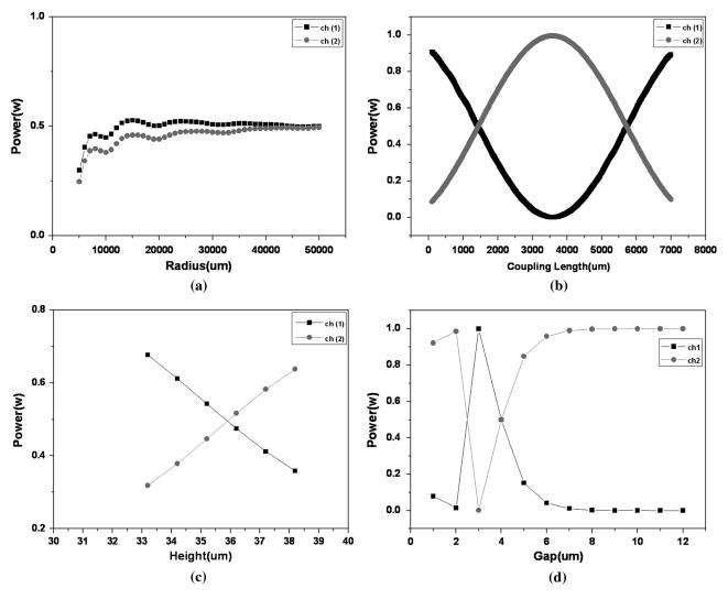
Fig. 2 Simulation results according to radius of curvature (a), coupling length (b), arm height (c), and gap of two waveguides (d).
