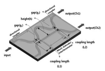
Fig. 1 The wavelength-independent coupler based on the Mach-Zehnder interferometer.
