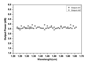
Fig. 8 Splitting characteristics according to wavelength.
