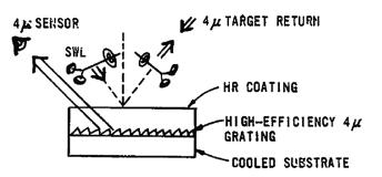
Fig. 13 A buried grating aperture sharing elements (ASE).
