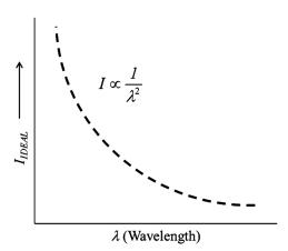
Fig. 2 Ideal short wavelength lasers (SWLs) far-field peak intensity.
