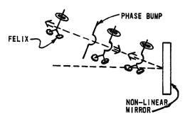
Fig. 21 Nonlinear optics (NLOs) mirror and aberrated beam.
