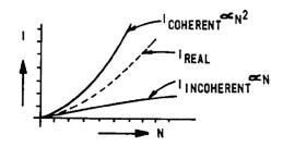
Fig. 18 Performance scaling of N coupled lasers.
