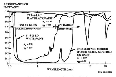
Fig. 16 Spectral absorptance for surfaces (Ref. 4).
