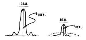
Fig. 7 Effects of short wavelength lasers (SWLs) phase aberrations on far-field performance.
