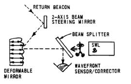
Fig. 17 Short wavelength lasers (SWL) adaptive optic (AO) systems.
