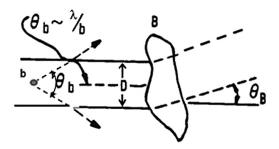
Fig. 3 Phase aberration effects on beam.
