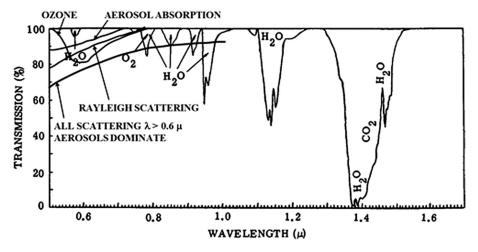
Fig. 14 Atmospheric scatter/absorption from molecular and aerosol constituents for sea level to space propagation (Ref. 2).
