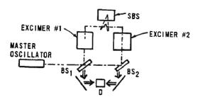
Fig. 24 Nonlinear adaptive optics (AO) application: coupled excimer lasers.
