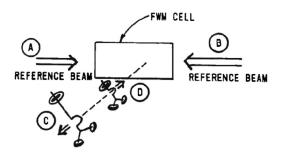
Fig. 23 Four wavelength mixing (FWM): an optical nonlinear process.
