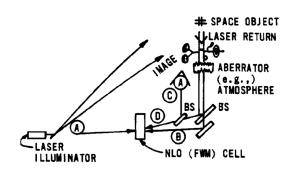
Fig. 28 One way image reconstruction via nonlinear optics (NLOs).
