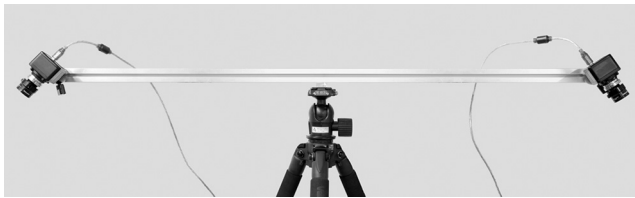
Fig. 6 The photo of two cameras system with nonoverlapped FOV.
