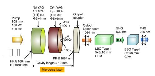
Fig. 1 Laser configuration with no intervening optics before nonlinear crystals.
