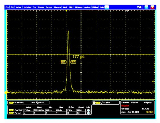
Fig. 4 Temporal profile of SHG output having a pulse width of 177 ps, measured using Tektronix DPO71604C oscilloscope and EOT ET-4000 detector.
