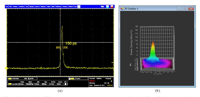
Fig. 5 (a) Temporal profile of FHG output having a pulse width of 177 ps, measured using Tektronix DPO71604C oscilloscope and Alphalas UPD-50-UD detector. (b) Beam profile of FHG pulse.
