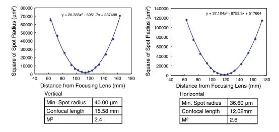
Fig. 6  $M^2$  measurement results for the output FHG beam.
