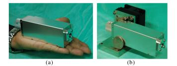
Fig. 2 Photograph of microlaser prototype without cooling (a) and with thermoelectric cooling (b).
